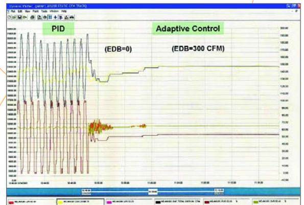
Actual comparison data between PID and Adaptive Control for air flow control at air handler, displayed in Dynamic Plotter at customer site.
