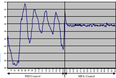
MFA (right) controls the key process variable much more tightly than PID (left).
