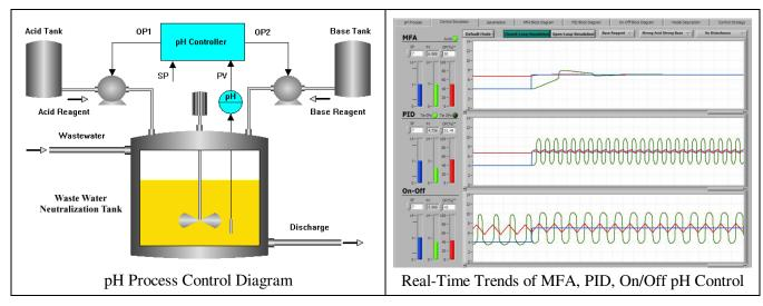
**pH Process:** Most process plants generate a wastewater effluent that must be neutralized prior to discharge or reuse. About 90% industrial wastewater pH processes are still controlled by On-Off control, resulting in chemical reagent wastes, equipment corrosion, and environmental pollution. Statistics show that a poorly controlled pH process can cost tens of thousands of dollars in chemical usage each month, not counting the penalties imposed by violating EPA or local discharge codes.
