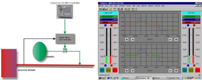
The trends compare MFA and PID control on the same strong-acid-strong-base pH processes. MFA (top) controls pH value tightly in all ranges at setpoint 7, 11, and 3. PID (bottom) is either sluggish or oscillating.
