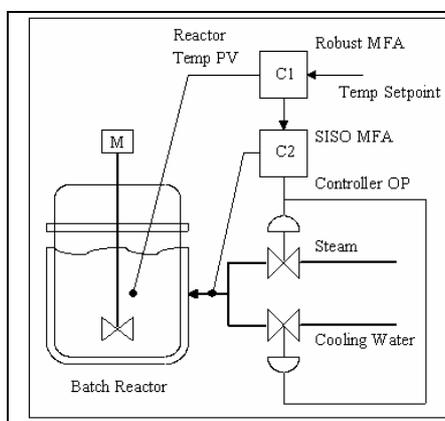
**Left:** Cascaded MFA control system with a Robust MFA as C1 to control reactor temp and a SISO MFA as C2 to control the steam and cooling water flow using the control output split-range design.
