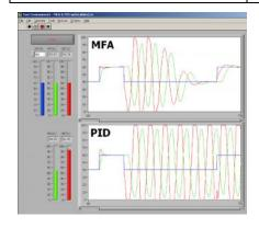
Left: When MFA (top) and PID (bottom) start from the same oscillating control condition, PID will continue to oscillate while MFA will quickly adapt to an excellent control condition. Both MFA and PID are running in a FieldPoint device.
