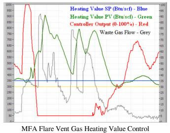
Flare Process: Most refinery and chemical plants operate flares to burn off waste gas. The vent gas heating value of a flare must be monitored and controlled based on EPA 40CFR60.18 rules.
