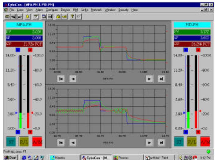
The trends compare MFA and PID control on the same strong-acid-strong-base pH processes. MFA (top) controls pH value tightly in all ranges at setpoint 7, 11, and 3. PID (bottom) is either sluggish or oscillating.
